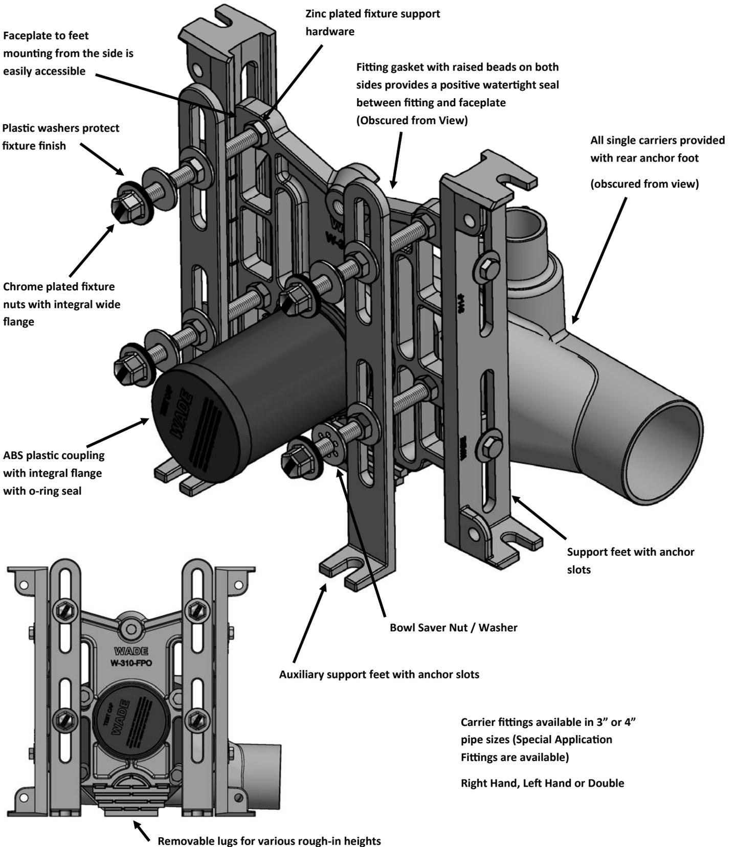
**311-XB Adjustable Horizontal Water Closet Carrier (1,000 Lb. Load Rating)**
