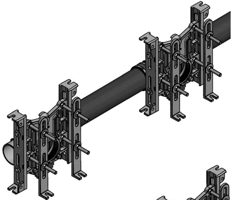
13. Coupling installation—Make sure the faceplate face is clean and free of debris. Insert O-Ring seal over threaded end of the coupling and lubricate with white petroleum jelly provided. Screw coupling into the 4" threaded boss on the front of the faceplate until the o-ring is sufficiently compressed.
