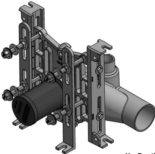
Bowl Saver Nut is provided to eliminate fixture flange damage. After three of the fixture nuts are tightened, use a nail or punch to screw the bowl saver nut into contact with the back of the fixture flange, then install the remaining chrome plated fixture nut and plastic washer.
