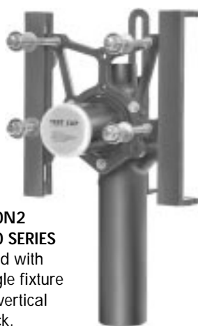
330NL 330 SERIES Used with single fixtures on common stack or in battery installations when horizontal waste is below the floor.
